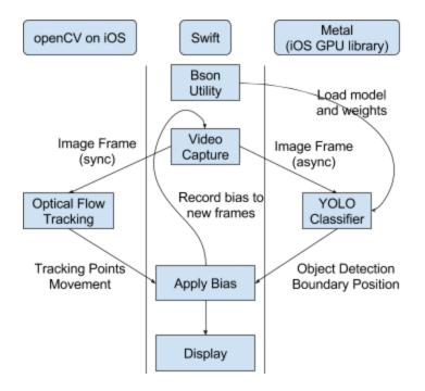
The above figure shows the general architecture of our project. We partially utilized an iOS based deep learning framework, which is written in swift, together with Metal to manipulate GPU computation resource. We also used OpenCV as an auxiliary method to smooth the detection experience.
