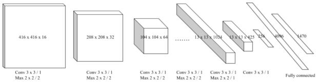
The above figure is the Tiny YOLO architecture we used.
